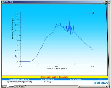
Above is an uncalibrated FluoroMax $^{\otimes}$  lamp-scan. The main peak ought to be at 467 nm, but here appears near 480 nm.
