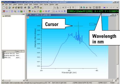
This example shows the peak at 477 nm, which is 10 nm too high. Therefore we must calibrate the monochromator.
